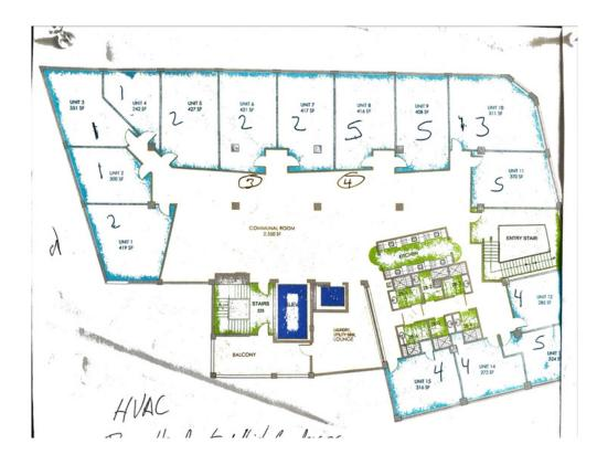
For AC to work in any of the apartments, all the apartments with corresponding system numbers on this map all have to have in room wall units must set to air-conditioning. Heating is the default, AC all has to be set consistent per connected heat pump system.
